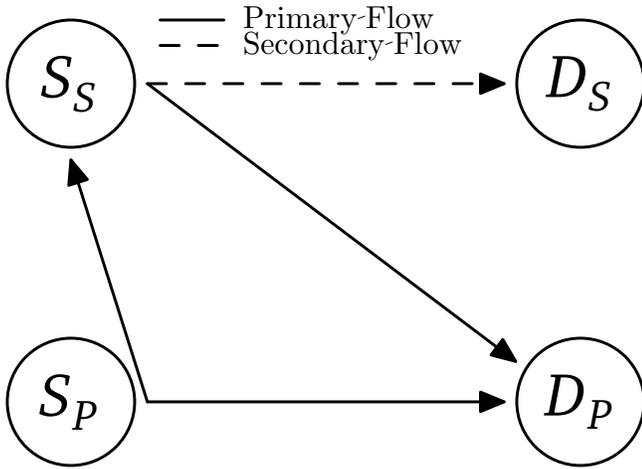
Figure 1. Wireless network with four nodes. If  $S_S$  is not present, the primary transmission from  $S_P$  to  $D_P$  occupies the entire medium.  $S_S$  can overhear the primary transmission and in some cases enhance it by relaying information. In such a case, resource gains may be shared with a secondary information flow from  $S_S$  to  $D_S$ , as a reward for cooperation.  $S_P$ , the spectrum owner, controls the whole process.
