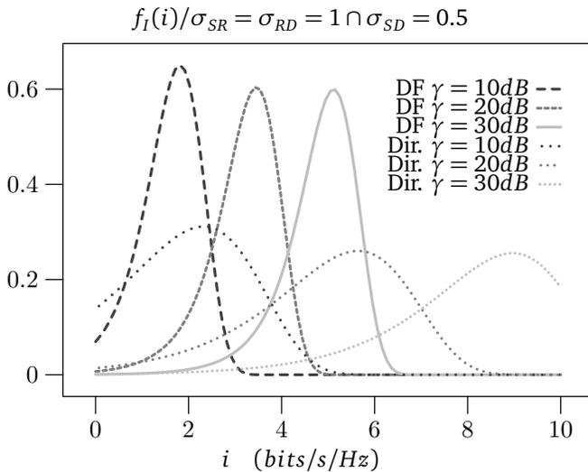
Figure 7. Mutual information p.d.f. of direct transmission and cooperative DF for the relay-in-the-middle layout. When the SNR is low, the p.d.f.s are highly overlapped. Thus, decisions based on instantaneous CSI would frequently switch between modes. DF lobes are still slightly shifted to the left compared to the respective direct transmission p.d.f.s. For higher SNRs the behavior is similar to that shown in figure 6.
