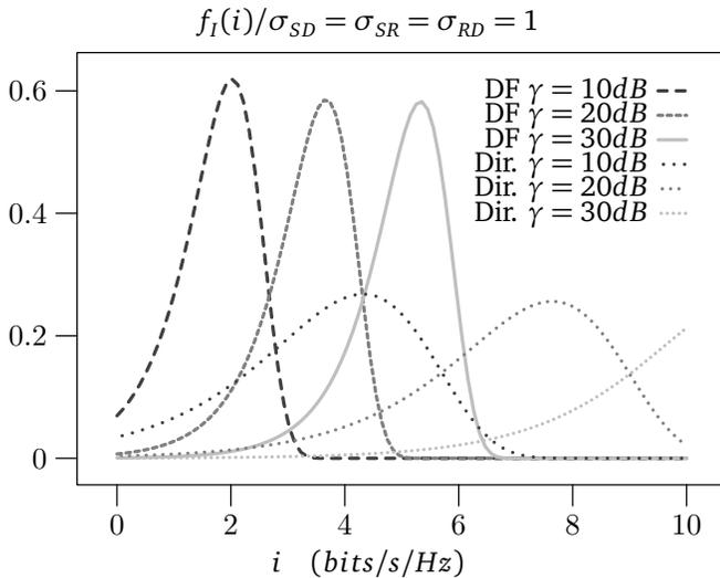
Figure 6. Mutual information p.d.f. of direct transmission and cooperative DF for the equilateral triangular layout. All DF p.d.f. lobes lie to the left of the corresponding direct transmission p.d.f.s. Decisions based on statistical CSI would select the direct mode and those based on instantaneous CSI would rarely opt for cooperative diversity when the direct channel is affected by deep fading.
